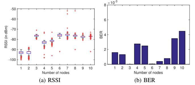
Fig. 9: RSSI and BER values in a model airliner fuselage with receiver at 10.5 m from concurrent transmitters.
