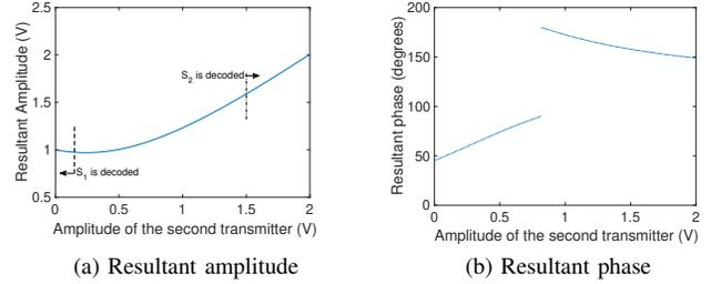
Fig. 6: Resultant amplitude and phase when  $A_1 = 1 \text{ V}$  and  $\phi_1 = \pi/4$ . Amplitude  $A_2$  is varied from  $0$  to  $2 \text{ V}$  in steps of  $0.01 \text{ V}$  and its phase is  $\phi_2 = 5\pi/6$ .
