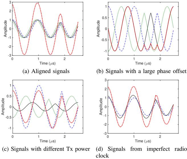
Fig. 1: The resultant signal (in red) when individual signals are aligned, have a temporal offset, have varying transmit powers and are subject clock errors on the radio.
