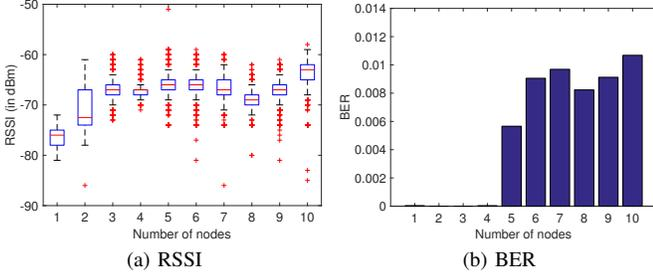
Fig. 8: RSSI and BER values in an empty office with receiver at 1 m from concurrent transmitters.
