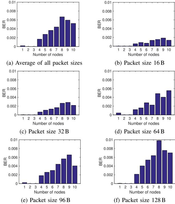
Fig. 12: BER in the soccer field for different packet sizes.
