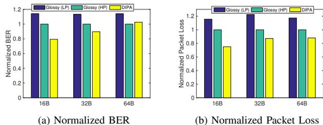
Fig. 15: Comparison between Glossy and Glossy with DIPA in w.iLab.t testbed.
