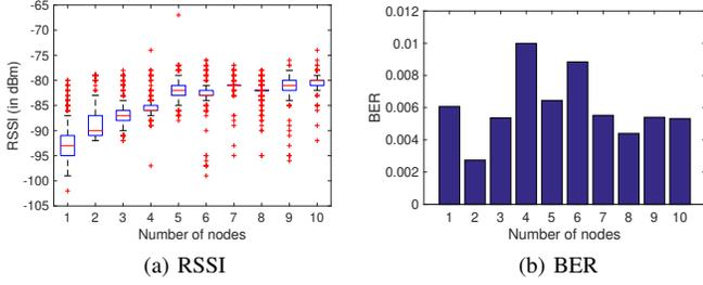
Fig. 7: RSSI and BER values in an empty office with receiver at 8 m from concurrent transmitters.
