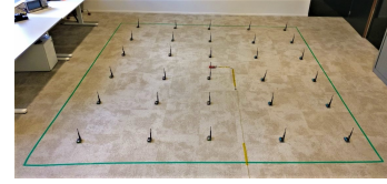
Fig. 12. A network of 30 SWITCHV3.0 nodes and gateway in a 4 m by 4 m area emulating multiple harvester events per second.
